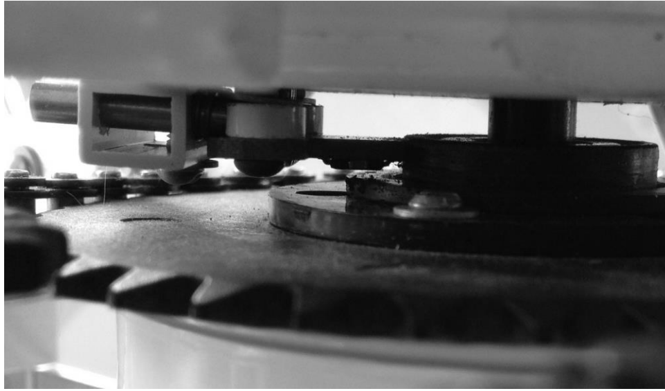
Figure 3.17. A close up shot of the encoder mounted just above a magnetic ring installed atop the main drive sprocket. The encoder package is mounted in a small custom PCB and the PCB is mounted on a spring loaded floating support cantilevered from a mount point located beneath the main chassis housing. The spring loaded support maintains the encoder sensor in proper position floating .5mm above the magnetic ring, and also allows for any rotational misalignment to be tolerated between the upper and lower chassis housings.
