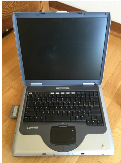
Figure 4.7. The Phase I detection target was an older laptop that we fitted with an 802.11g card supporting Linux raw wireless packet injection. The 802.11g card contained WLAN hardware built around the Atheros chipset.
