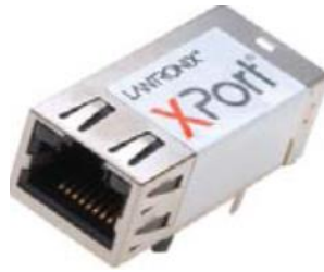
Figure 3.21. The XPORT 100mbps Serial-to-Ethernet Bridge. Limitations in the internal resonator clocking the master MCU keep serial communications speeds between MCU and bridge to a modest 38,400 BAUD.
